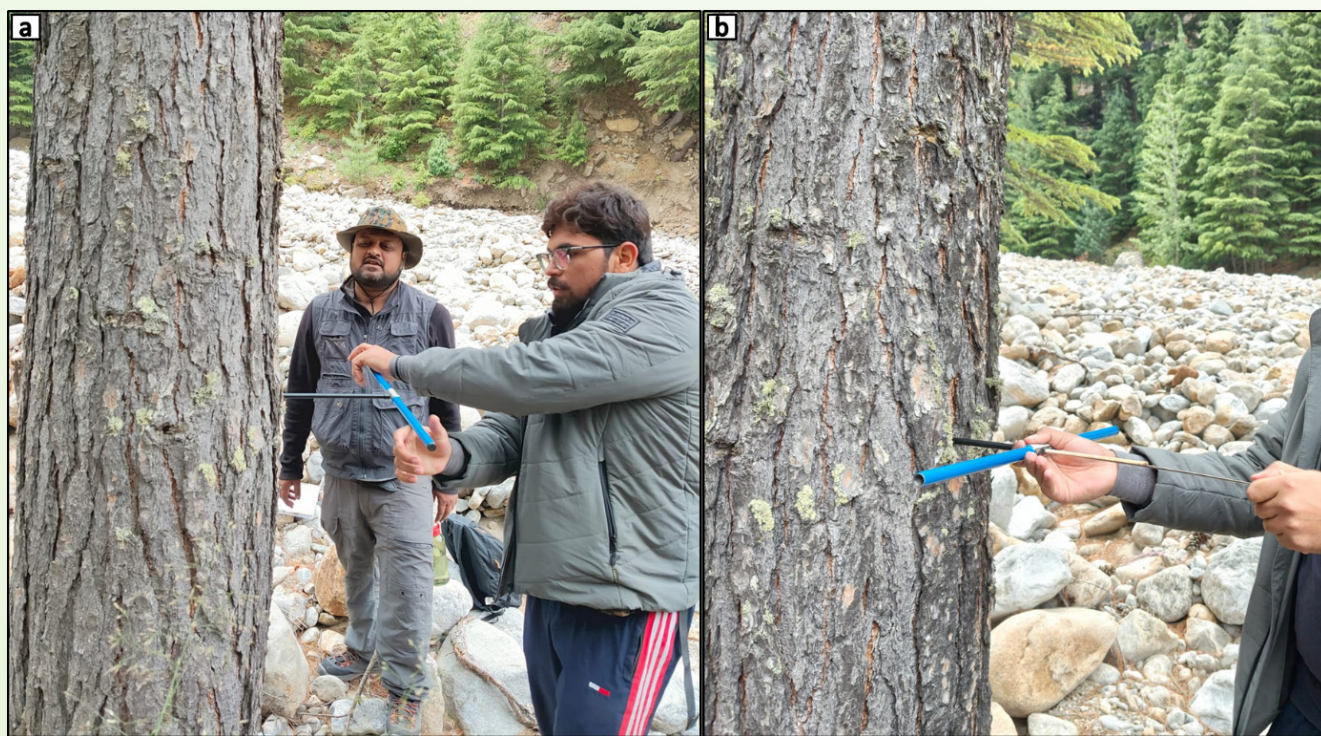
Figure. 2. Sample collection using an increment borer: (a) Boring into the tree stem, and (b) Retrieving the increment core using an extraction spoon.
